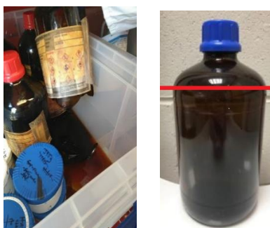
Figure 1 – Example of an incorrectly used Winchester and guide fill point
